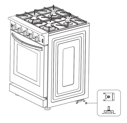
4 Open the storage drawer, slide the notches on the front brackets over the front feet, then screw the brackets into the floor using two of the provided screws for each bracket.
