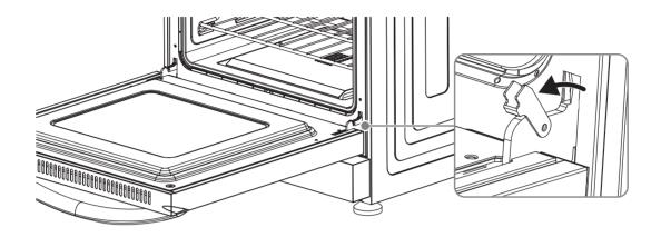
2 Gently close the door about halfway to disengage the hinges, then pull out the door and place it on a protected surface.
