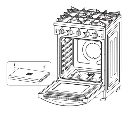
4 Remove the two screws from the pilot light and the single screw on the tube burner, then lift the lamp and burner up and out of the oven.
