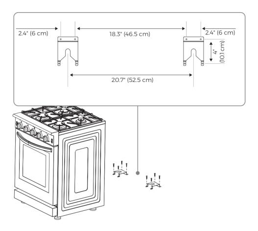
3 Align the rear feet with the notches on the rear brackets, then slide the range into place. Make sure that the rear feet are under the
