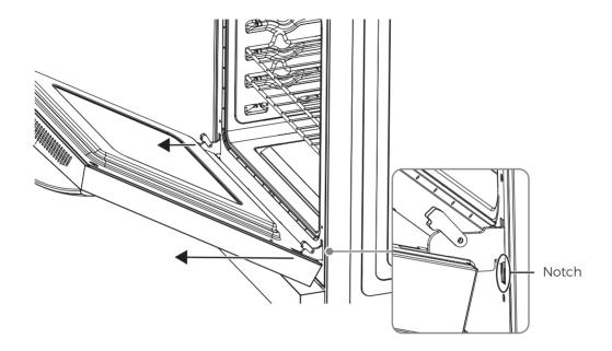
2 Carefully close the door. If the door does not easily close, do not force it. Make sure that the hinges are correctly installed.
